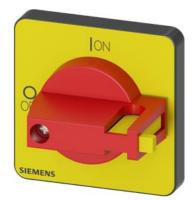
selector switch, red / yellow 48x48 mm Front plate mounting Central hole mounting 22.5mm for shaft 6x6 mm, accessory for Load disconnector 3LD3
